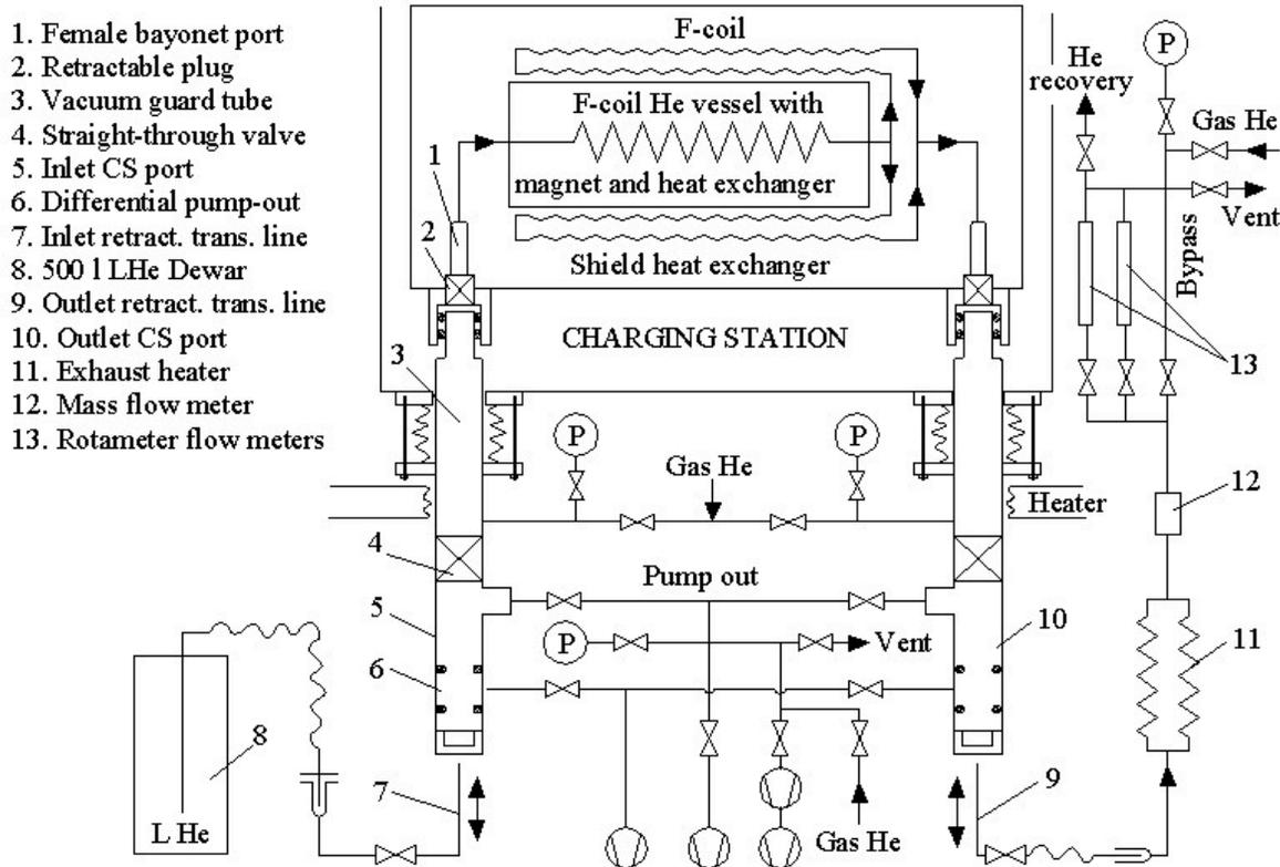
**FIGURE 1.** F-coil cooling, pumping out, and purging system (schematic). Transfer lines are retracted.
