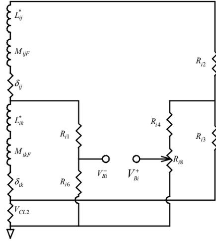
Fig. 4. Arrangement for the C-coil balance bridges.
