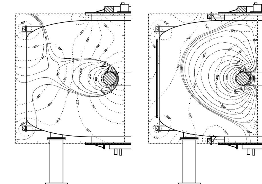
FIG. 2. The outer boundary of the levitated dipole plasma can be adjusted with low-field coils: (a) Outside diverted, (b) Inside diverted.
