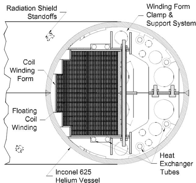
Fig.1. Helium vessel cross section.
