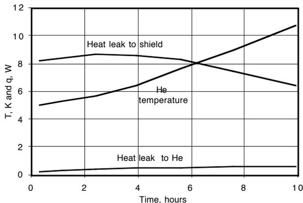
Fig. 3. Helium vessel and magnet temperature and heat leak in the cryostat.
