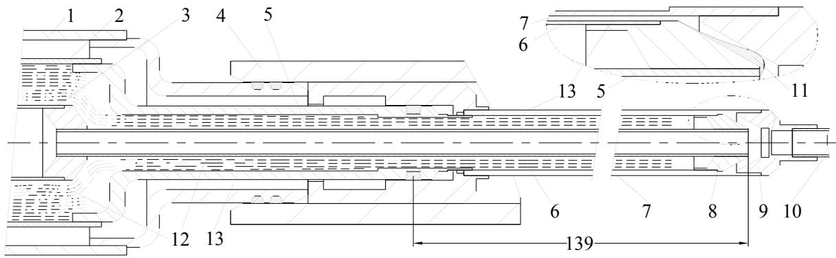
Figure 2 Transfer line bayonet joint. 1 – vacuum guard tube, 2 – vacuum jacket 28.6x0.9 mm, 3 – helium tube 9.53x0.7 mm, 4 – F-coil port, 5 – male part helium tube 4.76x0.4 mm, 6 – male part vacuum jacket 9.53x0.15 mm, 7 – female part tube 10.6x0.25 mm, 8 – male part tip, 9 - female part seat, 10 – F-coil heat exchanger tube, 11 - indium coating, 12 - MLI, 13 - vacuum
