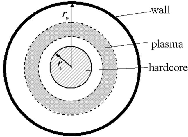
**Figure 3-1 Hardcore Z-pinch model of LDX**
