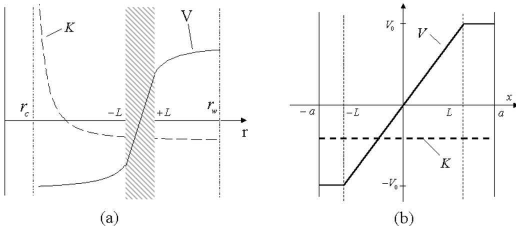
**Figure 3-6 (a) Cylindrical model showing a counter-streaming velocity profile in a region where  $K < 0$  (b) it's slab approximation**
