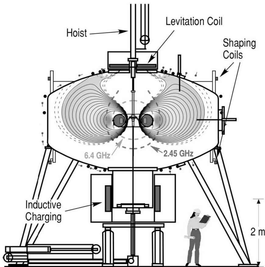
Figure 1-1 A schematics of the Levitated Dipole Experiment
