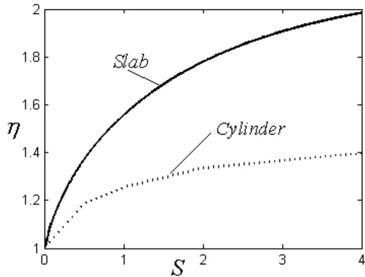
**Figure 3-12** The  $\beta$  ratio  $\eta$  vs. parameter  $S$  for slab predictions and actual cylindrical results
