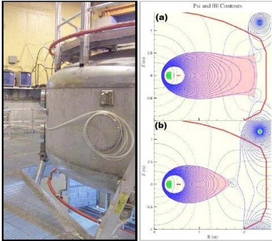
**Figure 2-1<sup>1</sup>** LHS- The LDX Helmholtz coils are shown above wrapped in red tape. RHS- The magnetic geometry for a Helmholtz field created with (a) 30 kA turns and (b) 50 kA turns.
