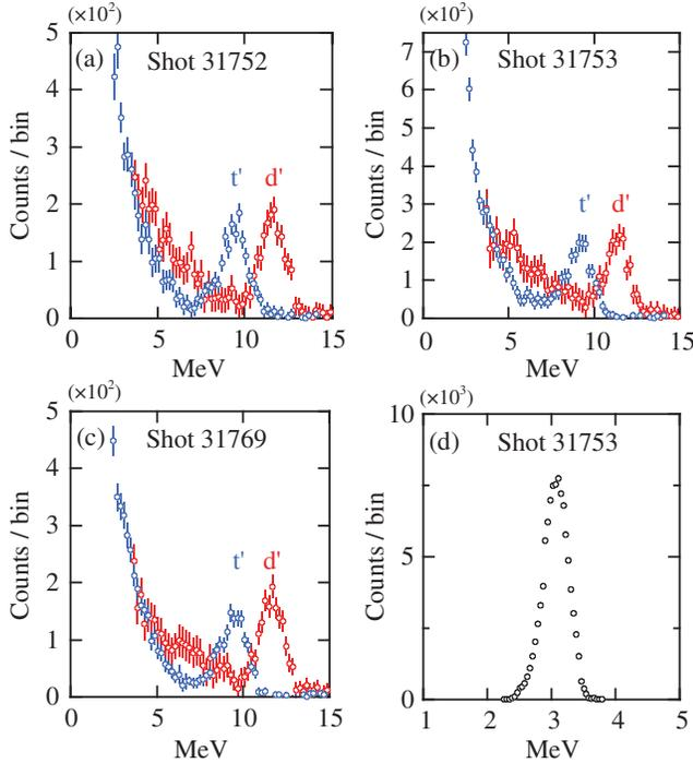
FIG. 2 (color). (a)–(c)  $d'$  and  $t'$  spectra measured simultaneously on three different OMEGA shots. The broadening of these spectra is due to the Doppler-effect and CPS-spectrometer response. (d)  $dd$ -proton spectrum measured for shot 31753 illustrates that the average energy is similar to the birth energy of 3.05 MeV.
