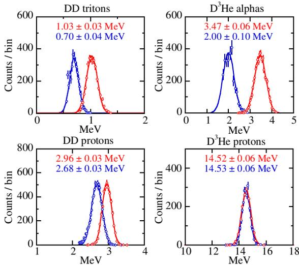
FIG. 1 (color online). CPS2-measured spectra of DD tritons,  $D^3He$  alphas, DD protons, and  $D^3He$  protons produced in implosions 29828 (blue) and 43233 (red). These experiments were designed to generate similar total  $\rho R$  values but to have most of the ion energy loss taking place in the cold remaining shell for implosion 29828 (blue spectra) and in the hot fuel for implosion 43233 (red spectra).
