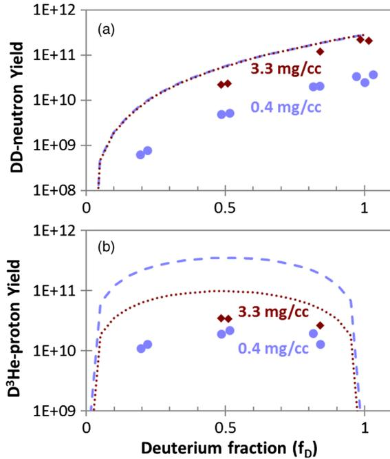
FIG. 1 (color online). Measured yields of (a) DD neutrons and (b)  $D^3He$  protons from implosions with initial fuel density of  $\rho_0 = 0.4$  (blue) and  $3.3$  (red) mg/cc. For each  $\rho_0$ , the deuterium fraction ( $f_D$ ) was varied. Points are artificially spread out in  $f_D$  for legibility. HYADES-simulated yield trends are shown for the low (dashed line) and high (dotted line)  $\rho_0$ .
