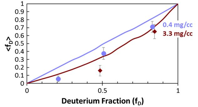
FIG. 4 (color online). “Burn-averaged deuterium fraction”  $\langle f_D \rangle$  evaluated from the experiments for low-density (blue) and high-density (red) implosions, compared to 1D-clean simulations (lines). Simulated values for  $\langle f_D \rangle$  differ slightly from the fuel  $f_D$  due to differences in the D $^3\text{He}$  and DD reactivity. Reduction of the deuterium in the core prior to burn is inferred for all implosions.
