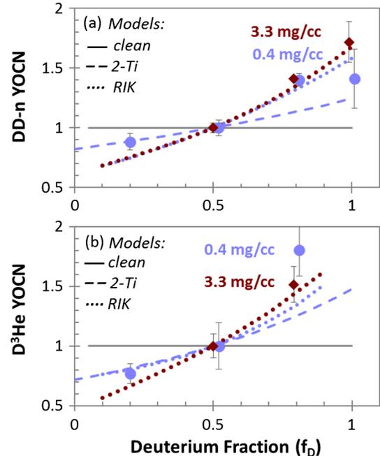
FIG. 2 (color online). Yields relative to clean 1D-HYADES simulations, for (a) DD neutrons and (b)  $D^3He$  protons. Each dataset has been normalized to its value at  $f_D = 0.5$ . Modeled trends incorporating kinetic physics, such as decoupled ion temperatures (“2-Ti”, dashed lines; low- $\rho_0$  only), and reduced ion kinetic models including ion diffusion (“RIK,” dotted lines) match the measurements better than clean simulations (solid lines).
