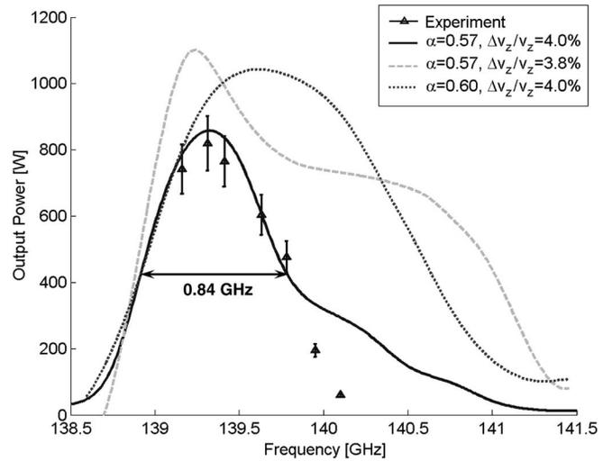
Fig. 8. Measured peak output power (markers) and simulations (curves) all at 37.7 kV and 2.7 A. The simulation fit is best for  $\alpha = 0.57$  and  $\delta v_z/v_z = 4.0\%$ . The experimental power has been measured at over 820 W.
