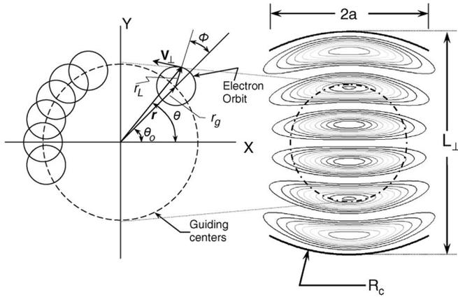
Fig. 1. (Left) Geometry of the electron beam showing guiding center beam radius  $r_g$  and Larmor radii  $r_L$ . (Right) Confocal interaction geometry showing mirror aperture half-width  $a$ , radii of curvature  $R_c$ , and mirror separation  $L_{\perp}$  with power contours for the  $HE_{06}$  mode superimposed. The electron beam interacts primarily with the second and fifth maxima.
