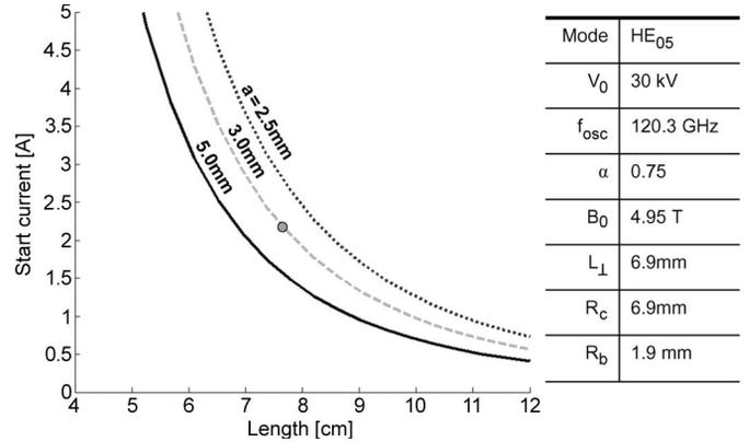
Fig. 4. Calculated BWO oscillation start current thresholds versus circuit length under the conditions shown for various mirror apertures  $a$ . The dot indicates that a 2-A beam current limits the circuit length to about 7.5 cm or less at 30 kV.
