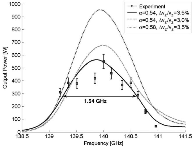
Fig. 7. Measured peak output power (markers) and simulations (curves) all at 38.5 kV and 2.5 A. The simulation fit is best for  $\alpha = 0.54$  and  $\delta v_z/v_z = 3.5\%$ . The experimental bandwidth has been measured at over 1.5 GHz.
