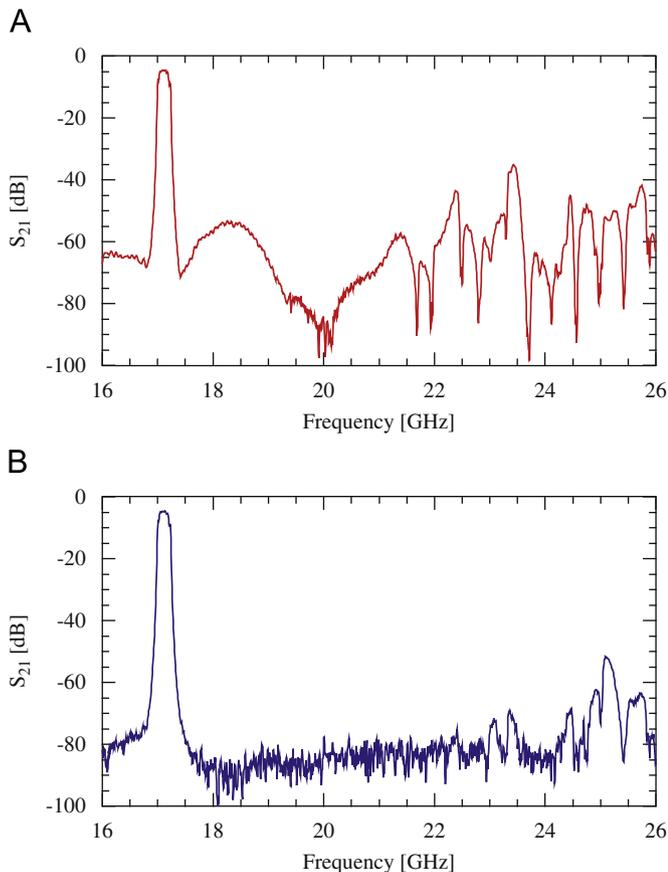
**Fig. 5.** Six cell metallic PBG accelerator structure uncalibrated  $S_{21}$  measurement. (A) is measured  $S_{21}$  without damping, (B) is measured  $S_{21}$  with external damping. Modes are observed at:  $\sim 17$ , and 23–27 GHz. Six modes are marginally resolved at 17 GHz, giving the resonances a broad appearance.
