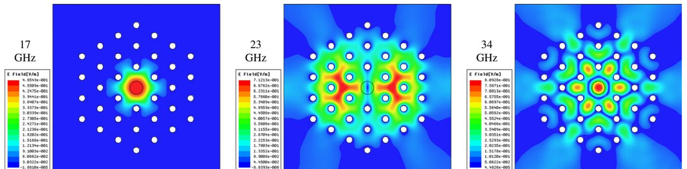
Fig. 4. HFSS simulations of 17, 23, and 34 GHz modes in one cell of the PBG accelerator structure. Irises and the outer boundary are bordered with PMLs, metallic rods and plates are modeled with ohmic losses. The electric field magnitude is shown in color. Simulation results correspond to the  $Q_{diffraction}$  runs as shown in Table 2.
