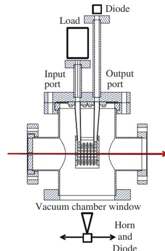
**Fig. 2.** PBG accelerator structure vacuum vessel. The waveguide input and output ports, and the chamber window on the bottom of the vacuum chamber are labeled. The positions of the matched load and diode detectors are shown. The beam path is indicated with a red arrow. (For interpretation of the references to color in this figure legend, the reader is referred to the web version of this article.)
