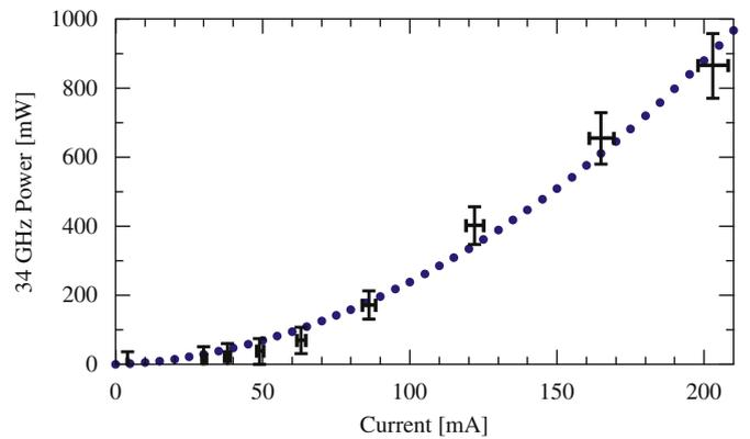
**Fig. 7.** Power observed on output port with matched input port, at 34 GHz, versus current. Quadratic fit to data shown as a dotted line with data given as bars.
