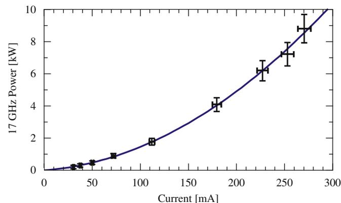
**Fig. 6.** Power observed on output port with matched input port, at 17 GHz, versus current. Theory prediction shown as a solid line with data given as bars.
