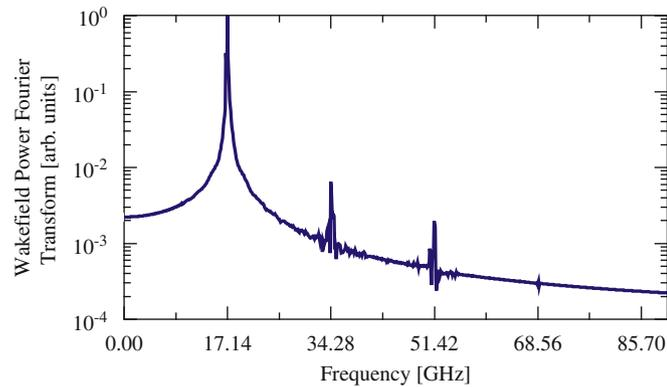
Fig. 3. Fourier transform of beam induced wakefield power versus frequency, as calculated using ANALYST for a 10 ps bunch length.
