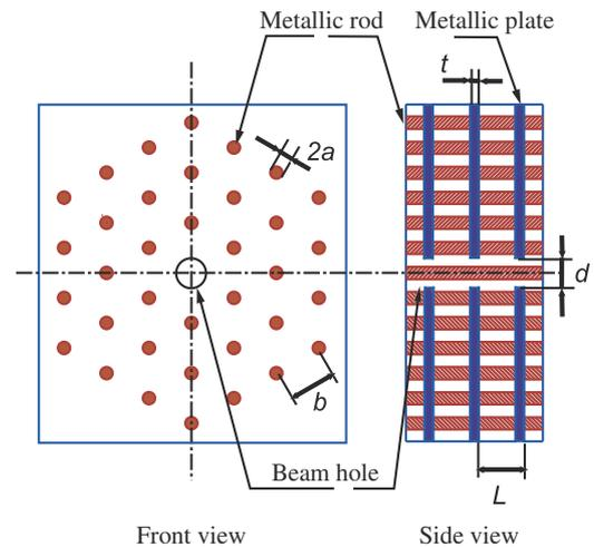
**Fig. 1.** Schematic of the six cell PBG accelerator structure. A PBG lattice is formed by a triangular lattice of cylindrical metallic rods; one rod is removed from the center to form a defect which confines the  $TM_{01}$  operating mode. Dimensions for labels are given in Table 1.
