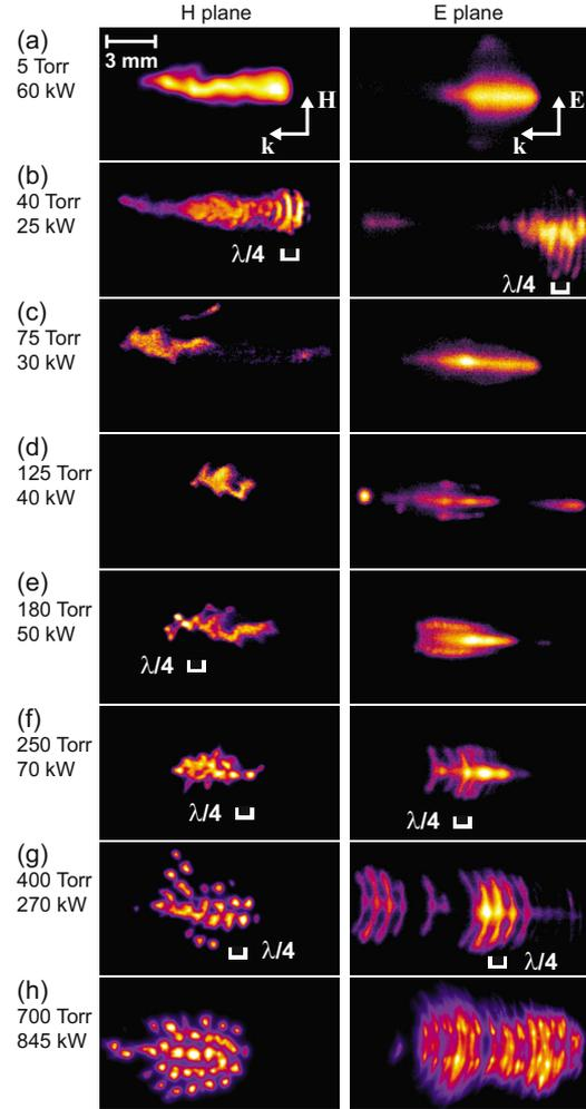
FIG. 2. (Color online) Breakdown in air, near threshold. (a) Diffuse plasma at 5 Torr. (b)  $\lambda/4$  structure appears at 40 Torr. [(c) and (d)] Plasma fans out in H plane. [(e) and (f)] Triangular array appears in H plane. [(g) and (h)] Clear filament array is fully developed at high pressure.
