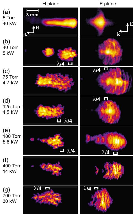
FIG. 3. (Color online) Breakdown in argon, near threshold. (a) Diffuse plasma at 5 Torr. (b)  $\lambda/4$  structure appears at 40 Torr. [(c)–(e)]  $\lambda/4$  structure becomes sharper. [(f)–(g)] Plasma structure is well-defined at high pressure.
