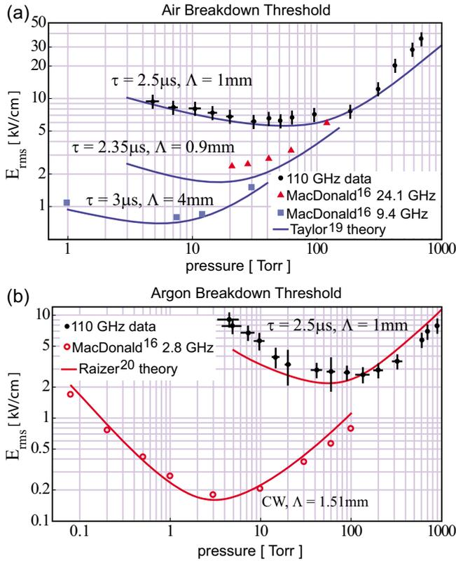
FIG. 1. (Color online) Breakdown threshold field vs pressure. (a) Air data: 110 GHz (circles), MacDonalD 24.1 GHz (triangles), MacDonalD 9.4 GHz (squares), Taylor model (curve). (b) Argon data: 110 GHz (circles), MacDonalD 2.8 GHz (open circles), Raizer model (curve).
