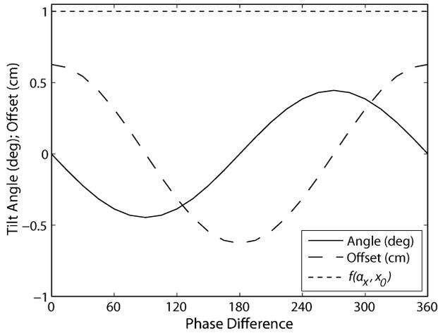
Fig. 11. Centroid offset and tilt angle for an input of 90%  $HE_{11}$  and 10%  $LP_{11}^{(e)}$  in a waveguide of radius  $a = 31.75$  mm at 170 GHz.  $f(\alpha_x, x_0)$  plots (36). A  $2\pi$  phase difference corresponds to  $z_1 = 5.07$  m.
