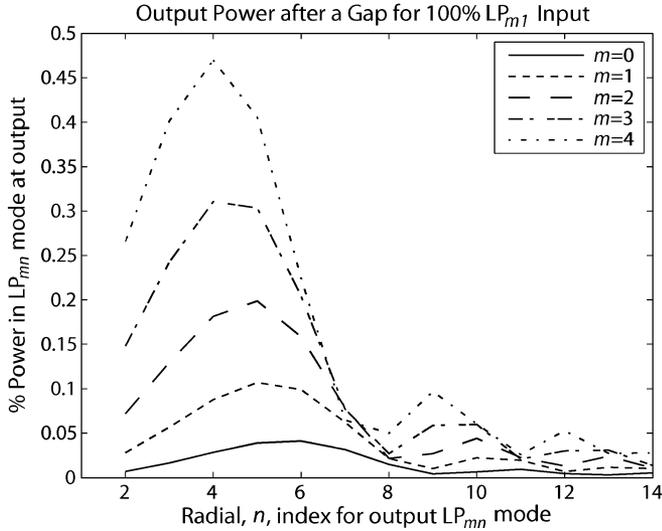
Fig. 5. Percent output of the power present in the  $LP_{mn}$  modes after a gap that results from a 100%  $LP_{m1}$  mode input, for  $m = 0-4$ .  $LP_{m1}$  mode power outputs (which are over 94%) have been cropped to emphasize higher order mode contents.
