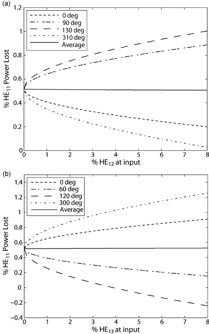
Fig. 6. For a two-mode input at 170 GHz with  $a = 31.75$  mm and  $L = 2a$ , the percent of (a) HE<sub>12</sub> or (b) HE<sub>13</sub> present in the input mode mixture versus the percent loss in HE<sub>11</sub> after the gap is plotted. Different phases of HE<sub>12</sub> or HE<sub>13</sub> have been chosen to show the full range of swing in the HE<sub>11</sub> power loss. The average HE<sub>11</sub> power loss is 0.52% for both cases.
