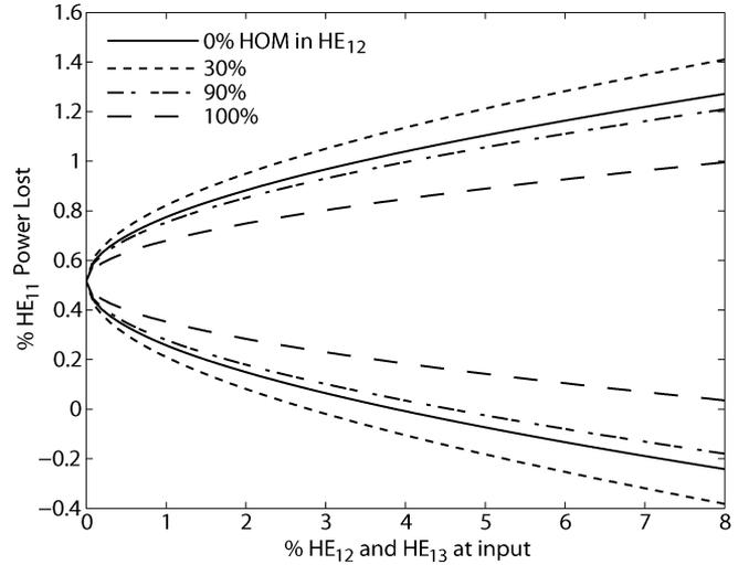
Fig. 7. Power loss in a gap for HE<sub>11</sub> versus higher order mode content for a three-mode input. The higher order mode content is split between HE<sub>12</sub> and HE<sub>13</sub>, and the largest and smallest HE<sub>11</sub> power loss (due to higher order mode phase) is plotted for each mode split. The system is at 170 GHz with  $a = 31.75$  mm.
