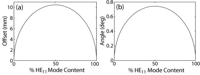
Fig. 9. Maximum: (a) offset and (b) tilt angle versus HE<sub>11</sub> percent content [ $A_p$  in (20)] for a combination of HE<sub>11</sub> and LP<sub>11</sub> modes.
