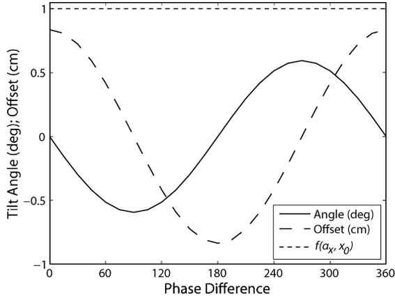
Fig. 10. Centroid offset and tilt angle for an input of 80%  $HE_{11}$  and 20%  $LP_{11}^{(e)}$  in a waveguide of radius  $a = 31.75$  mm at 170 GHz.  $f(\alpha_x, x_0)$  plots (36). A  $2\pi$  phase difference corresponds to  $z_1 = 5.07$  m.
