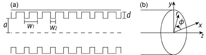
Fig. 1. (a) Cylindrical circumferentially corrugated waveguide with a radius of  $a$ . The corrugations are defined by  $w_1$ ,  $w_2$ , and  $d$ . For low-loss characteristics, the corrugation depth is  $d = \lambda/4$ . (b) Illustration of the variables in the cylindrical geometry.
