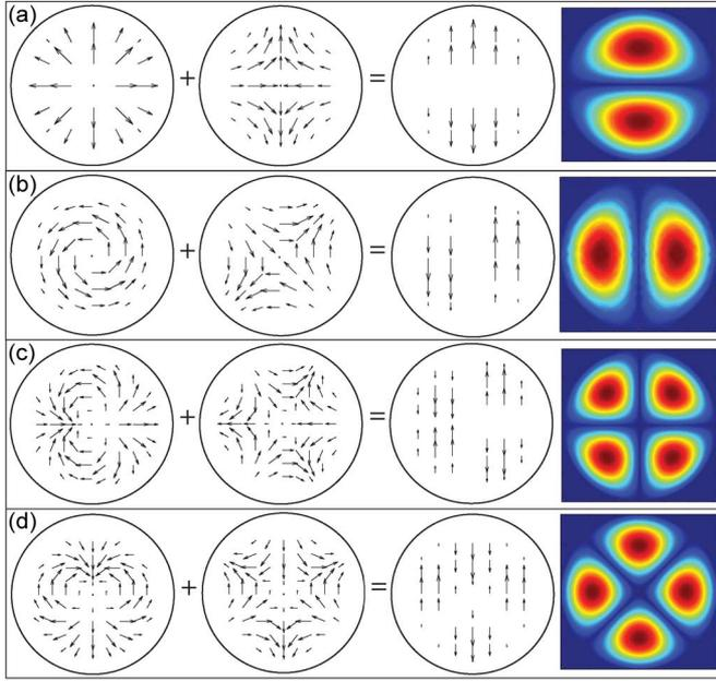
Fig. 3. Field vector plots demonstrating the construction of LP modes from TE, TM, and HE modes. The added modes have identical propagation constants. (a)  $TM_{02} + HE_{21}$  rotated  $45^\circ = LP_{11}^{(e)}$ . (b)  $-TE_{01} + HE_{21} = LP_{11}^{(o)}$ . (c)  $EH_{12}$  rotated  $-90^\circ + HE_{31}$  rotated  $-90^\circ = LP_{21}^{(e)}$ . (d)  $EH_{12}$  rotated  $180^\circ + HE_{31} = LP_{21}^{(o)}$ .
