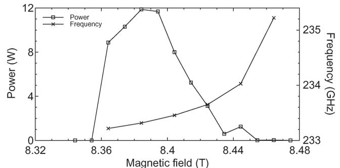
Fig. 6. CW output power and frequency in the  $TE_{2,3,q}$  modes as a function of magnetic field for 50 mA and 3.5 kV.
