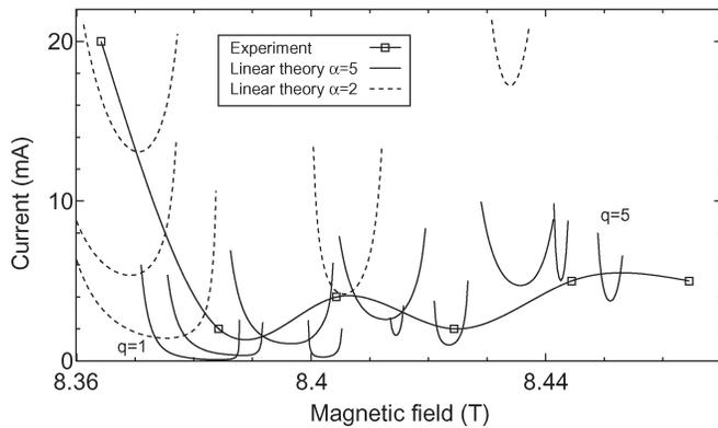
Fig. 4. CW start current data in the  $TE_{2,3,q}$  series of axial modes at 3.5 kV compared to linear theory using  $\alpha$  equal to two and five and with 12% transverse velocity spread.
