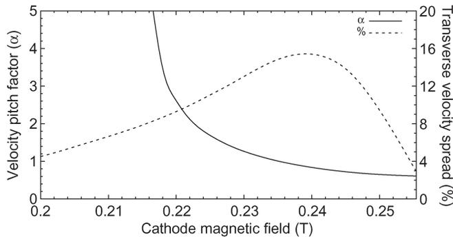
Fig. 3. Electron-gun simulation using EGUN electron optics code of the velocity-pitch factor (solid line) and transverse velocity spread (dashed line) for 10 mA, 3.5 kV, and 8.38 T.
