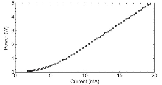
Fig. 2. CW output power in the  $TE_{2,3,1}$  mode as a function of beam current at 3.5 kV and 8.38 T.
