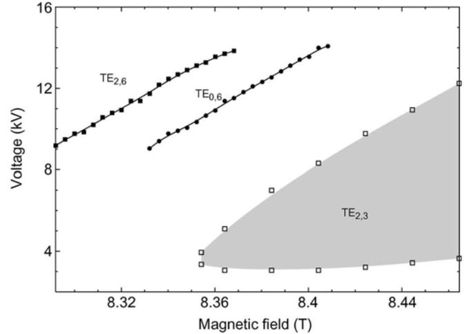
Fig. 1. Mode excitation regions for two second-harmonic modes ( $TE_{2,6}$  and  $TE_{0,6}$ ) and nearby fundamental harmonic mode ( $TE_{2,3}$ ) over beam voltage, cavity, and, implicitly, cathode magnetic fields.
