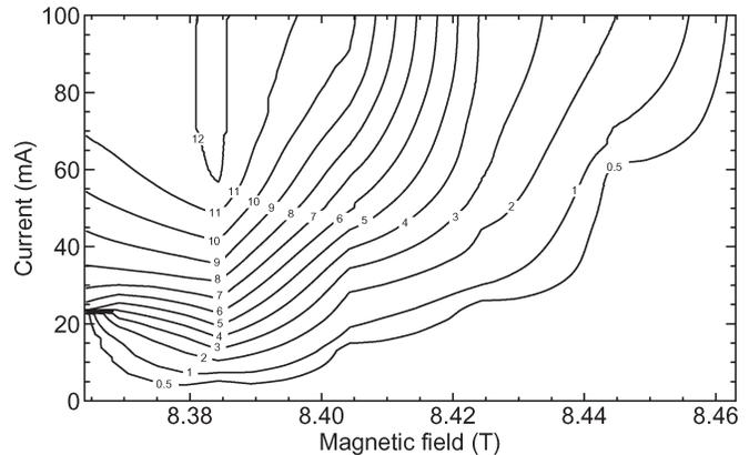
Fig. 5. Contour plot of measured CW power data of the fundamental harmonic  $TE_{2,3,q}$  modes in watts as a function of beam current and magnetic field for an electron-beam voltage of 3.5 kV.
