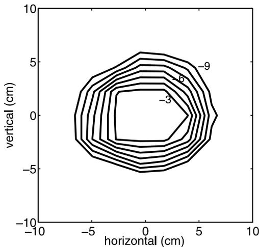
Fig. 2. Plot of the measured power of the Gaussian-like output beam at 73.6 cm from the window location along the output beam axis. The contours represent the intensity of the beam in dB between 3 and 9 dB down from the peak. Horizontal: parallel to the gyrotron axis; vertical: perpendicular to the gyrotron axis.
