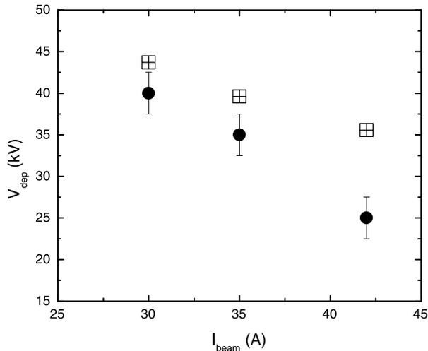
Fig. 7. A threshold collector depression voltage as a function of beam current at 96.6 kV of beam voltage. Circles with error bars represent experimental measurements, and crossed-squares represent the simulation results.
