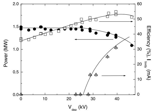
Fig. 6. Power, efficiency, and body current measurements as a function of depression voltage of the collector. Solid circles: output power; open squares: an efficiency plot; and open triangles: a body current plot.
