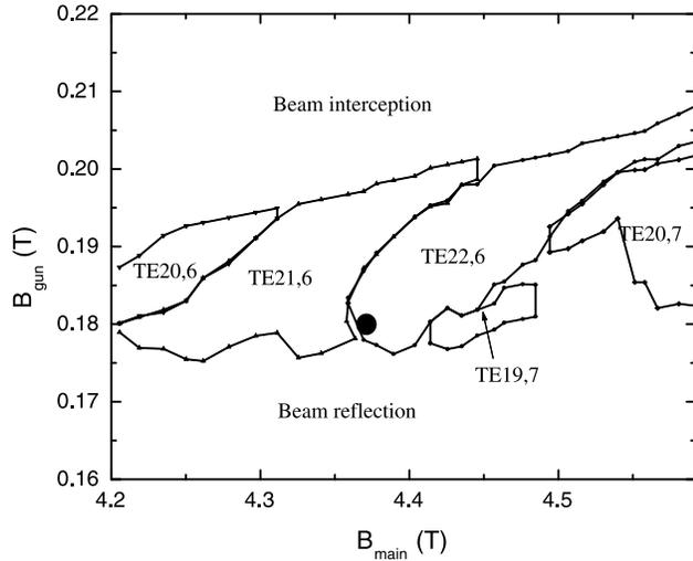
Fig. 4. Mode map plot in the IMC configuration measured at 96.6 kV of beam voltage and 42 A of current. The circle indicates the maximum power point.
