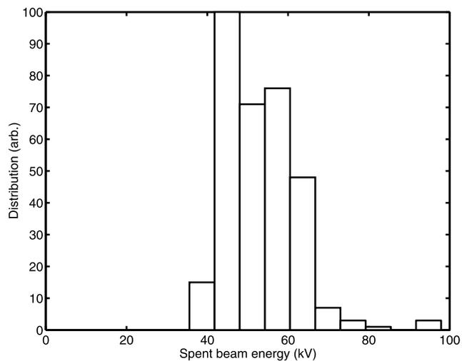
Fig. 8. Distribution of the spent energy of the electron beam at 42 A of beam current and 1.5 MW of output power. The number of electron beamlets used in the calculation was 81.
