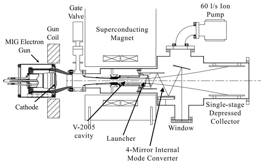
Fig. 1. The 1.5-MW, 110-GHz gyrotron schematic.
