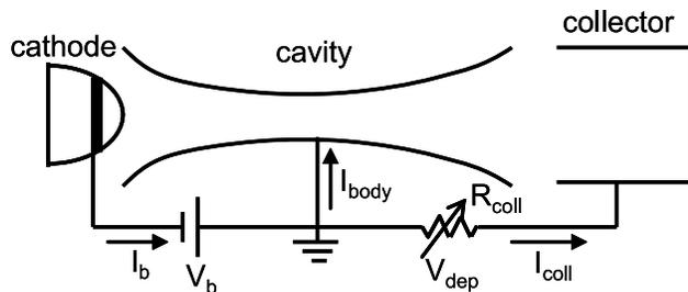
Fig. 5. A circuit schematic for the single-stage depressed collector.
