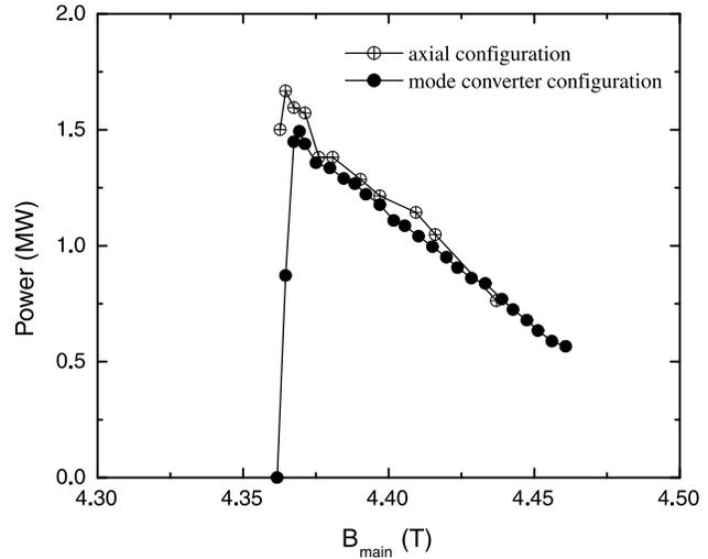
Fig. 3. Power measurement as a function of main magnetic field at 96.6 kV of beam voltage and 42 A of beam current. Open circles represent the axial configuration results, and solid circles represent the IMC configuration.
