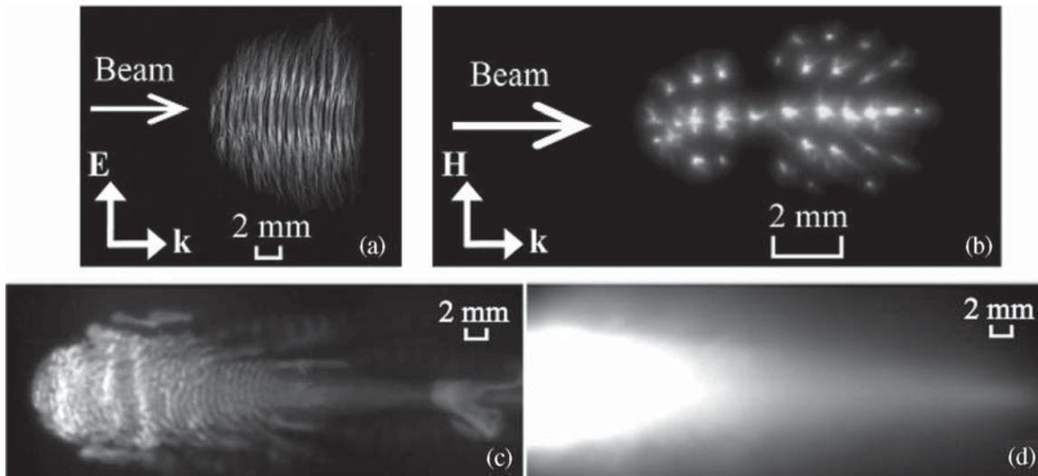
Fig. 1. Time-integrated images of air plasma in (a) E-plane at 760 torr and (b)–(d) H-plane at 760, 50, and 0.7 torr, respectively. The camera sensor is exposed during the entire microwave pulselength. Camera sensor gain settings are different in each shot. The light emission intensity decreases as pressure decreases.
