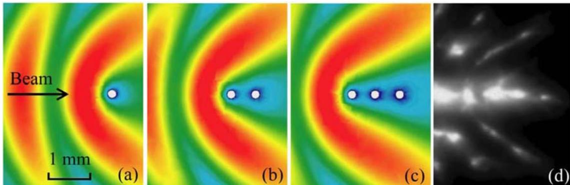
Fig. 2. Simulation results of total E-field magnitude with (a) one, (b) two, and (c) three plasma filaments modeled as (white circles) perfectly conducting metal posts. (d) Volume breakdown image at atmospheric pressure in H-plane.
