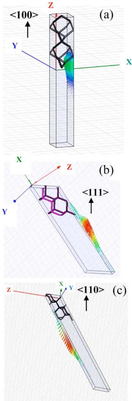
FIG. 6. (Color online) Stack of cells used for surface mode simulation on (a) the anisotropic (100) interface, (b) isotropic (111) interface, and (c) anisotropic (110) interface. The electric field distribution in the surface modes is shown.
