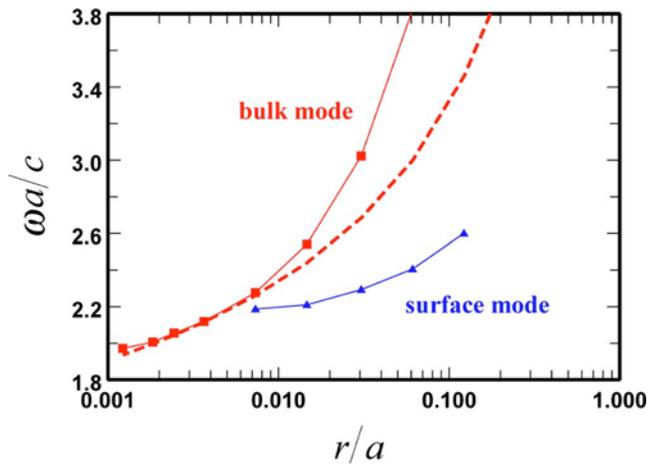
FIG. 3. (Color online) Normalized plasma frequency of bulk modes as a function of the ratio of rod radius  $r$  to cubic cell length  $a$  (red solid line), analytical representation of Eq. (1) (dashed line), and normalized resonance frequency of the surface mode on the anisotropic (100) interface (blue line).
