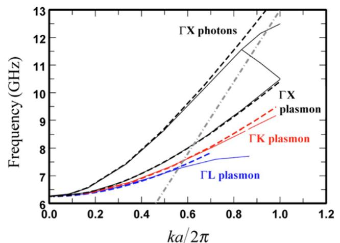
FIG. 5. (Color online) Comparison of wave dispersion in the lattice (solid lines) and the SD medium (dashed lines):  $\Gamma$ - $X$  plasmon and photons (black),  $\Gamma$ - $L$  plasmon (blue), and  $\Gamma$ - $K$  plasmon (red).
