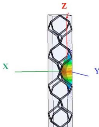
FIG. 9. (Color online) Simulation of plasmonic waveguide. The defect mode is a longitudinal TM mode propagating in the  $x$ -direction. The electric field distribution is shown.
