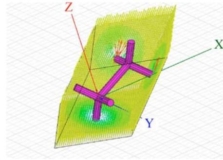
FIG. 2. (Color online) Simulation of bulk modes in the diamond wire lattice using the primitive cell. A longitudinal plasma mode at 6.25 GHz is shown for the lattice cubic cell length  $a=2.3$  cm and the wire radius  $r=0.07$  cm.
