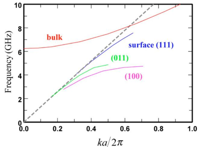
FIG. 7. (Color online) Dispersion of bulk waves and surface waves on the isotropic interface (111) and anisotropic interfaces (100) and (011) of the diamond metallic lattice. The cubic cell period is  $a = 2.3$  cm and wire radius  $r = 0.07$  cm. The dashed line depicts the light dispersion in vacuum. The frequency of the isotropic (111) interface mode tends to the plasma frequency, which disagrees with the “artificial plasma” model.
