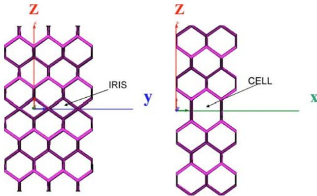
FIG. 8. (Color online) Accelerator structure using a defect in 3D metallic diamond wire lattice. An electron beam traverses in the  $x$ -direction.
