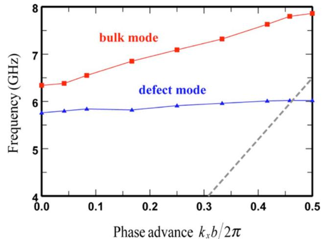
FIG. 10. (Color online) Dispersion of plasmonic waveguide modes. The defect mode is an accelerating mode. Dashed line is the light dispersion in vacuum. The cubic cell length  $a=2.3$  cm and wire radius  $r=0.07$  cm.
