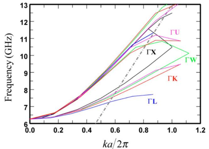
FIG. 4. (Color online) Dispersion of longitudinal (plasmon) and transverse (photon) waves. One plasmon and two photons are calculated for each of the following directions:  $\Gamma$ - $X$  (black),  $\Gamma$ - $W$  (green),  $\Gamma$ - $U$  (magenta),  $\Gamma$ - $K$  (red), and  $\Gamma$ - $L$  (blue). Dashed-dotted straight line is the light dispersion in vacuum.
