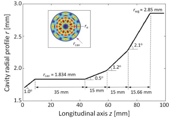
Fig. 2. Schematic of the 330-GHz gyrotron interaction circuit. The inset shows the transverse electric field profile of the cavity mode  $TE_{-4,3}$  and the location of the electron beam with radius  $r_e = 1.08$  mm.
