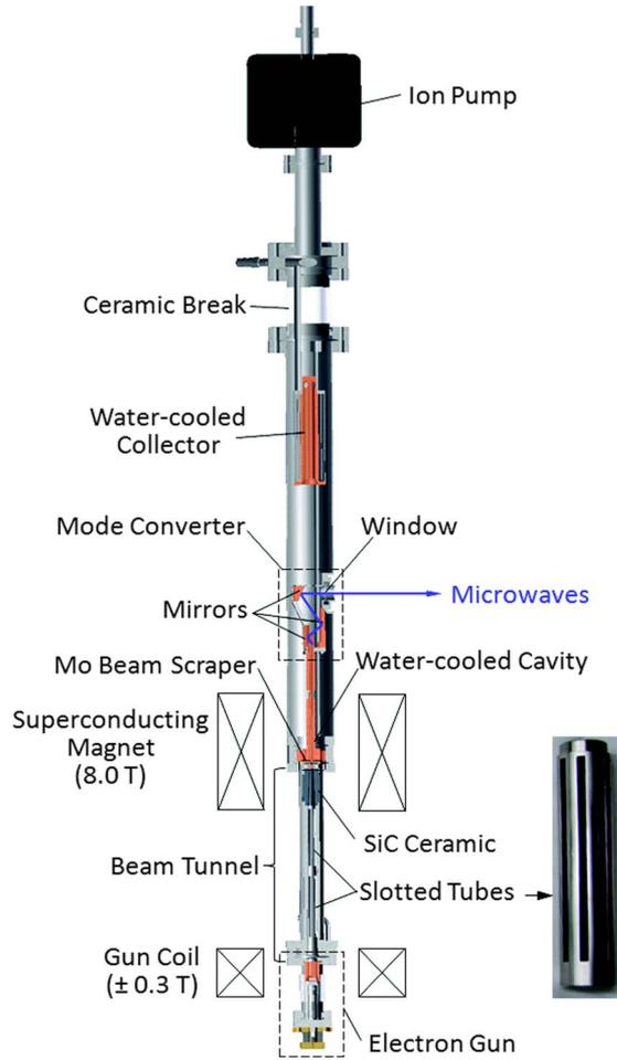
Fig. 1. Schematic of the 330-GHz gyrotron oscillator. A picture of a slotted tube utilized in the gyrotron beam tunnel is also shown.
