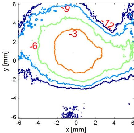
Fig. 11. Gyrotron output microwave beam pattern captured by a pyroelectric camera after the end of the corrugated waveguide. The beam pattern is displayed in decibel contours. Gyrotron parameters: Magnetic field  $B_0 = 6.003$  T, beam voltage  $V_b = 9.6$  kV, beam current  $I_b = 32$  mA, frequency = 330.17 GHz, and output power of 0.4 W.
