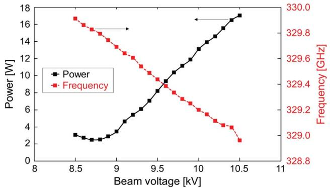
Fig. 7. (Solid line) Power and (dashed line) frequency tuning measurements as a function of beam voltage for magnetic field  $B_0 = 6.003$  T, beam current  $I_b = 190$  mA, and cavity cooling channel temperature  $T_{water} = 9$  °C. The gun coil was swept from  $B_{gun} = 1$  mT to  $B_{gun} = -25$  mT for the best output power as the beam voltage was decreased.
