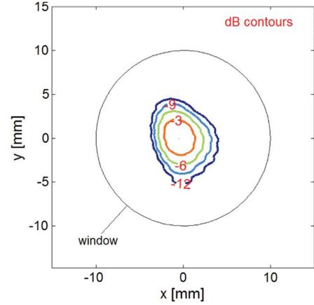
Fig. 4. Simulated electric field of 330-GHz microwave output beam at the focal plane. The beam pattern is displayed in decibel contours. The gyrotron window is shown as reference.
