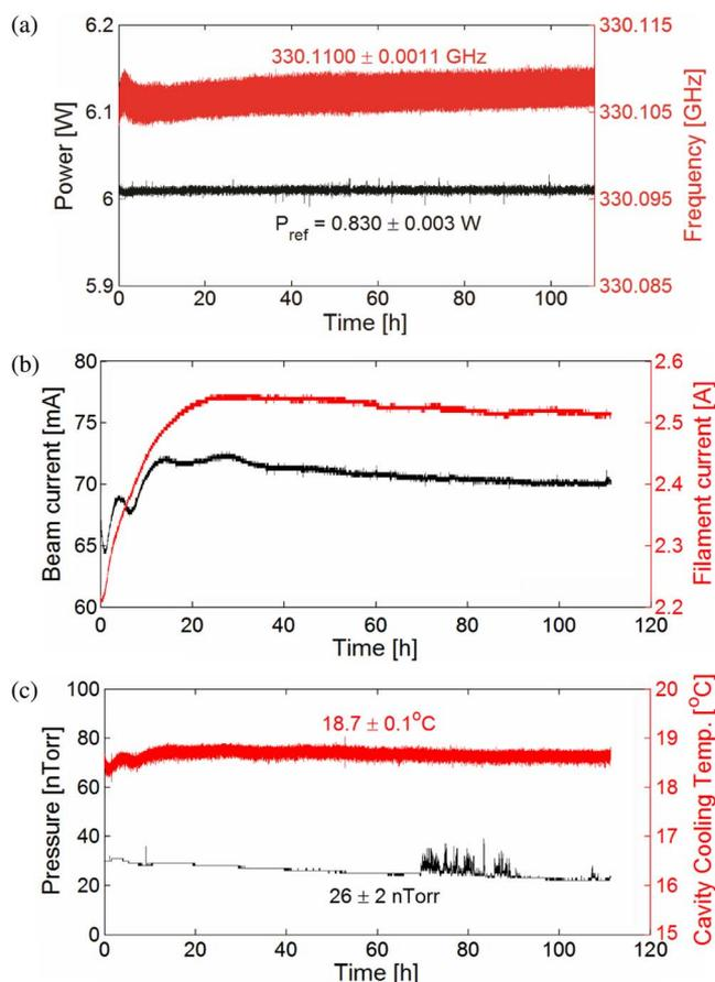
Fig. 10. Monitored variables during the CW long-run stability test of the 330-GHz second-harmonic gyrotron: (a) Output power and frequency, (b) beam and cathode filament currents, and (c) pressure and cavity cooling temperature. During the test, the magnetic field was persistent at  $B_0 = 6.006$  T, and the beam voltage was fixed at  $V_b = 10.0$  kV.
