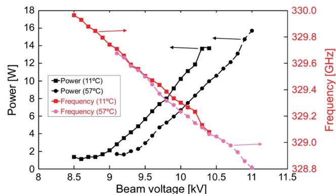
Fig. 9. Voltage tuning measurement for magnetic field  $B_0 = 6.003$  T, beam current  $I_b = 150$  mA, as well as the cavity cooling channel temperatures (square markers)  $T_{\text{water}} = 11$  °C and (circular markers)  $T_{\text{water}} = 57$  °C.
