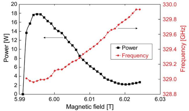
Fig. 6. (Solid line) Power and (dashed line) frequency tuning measurements as a function of magnetic field for beam voltage  $V_b = 10.1$  kV, beam current  $I_b = 190$  mA, and cavity cooling channel temperature  $T_{water} = 9$  °C. The gun coil was swept from  $B_{gun} = -3$  mT to  $B_{gun} = -5$  mT for the best output power as the magnetic field was increased.
