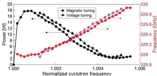
Fig. 8. (Circular marks) Magnetic and (diamond marks) voltage tuning measurements for beam current  $I_b = 190$  mA and cavity cooling channel temperature  $T_{\text{water}} = 9$  °C. The magnetic and voltage tuning data were taken at  $V_b = 10.1$  kV and  $B_0 = 6.003$  T, respectively.
