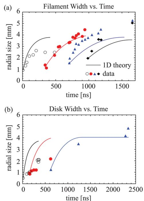
FIG. 6. (Color online) Radial size of (a) filaments (linear polarization) and (b) disks (circular polarization) vs. camera trigger time,  $t$ , for plasmas born at different times.
