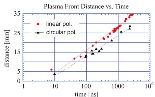
FIG. 4. (Color online) Position of the plasma front vs. camera trigger time  $t$ . The lines are logarithmic fits to the data.
