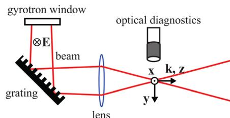
FIG. 1. (Color online) Experimental setup: The breakdown plasma initiates at the origin of the coordinate system at the center of the focused beam waist.
