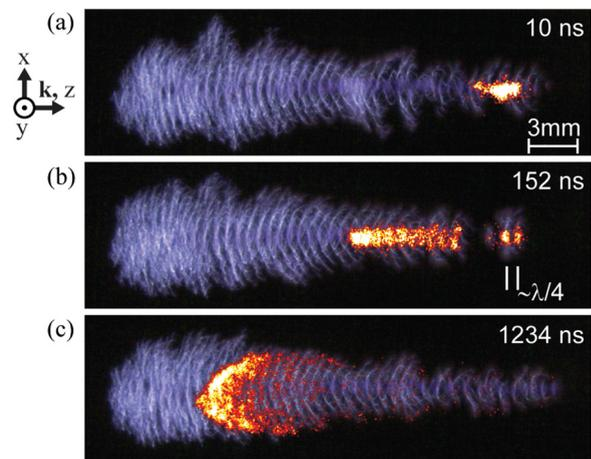
FIG. 3. (Color online) Open-shutter (background image, blue) and fast-gated (overlay, orange) photographs of breakdowns with circularly polarized beam.
