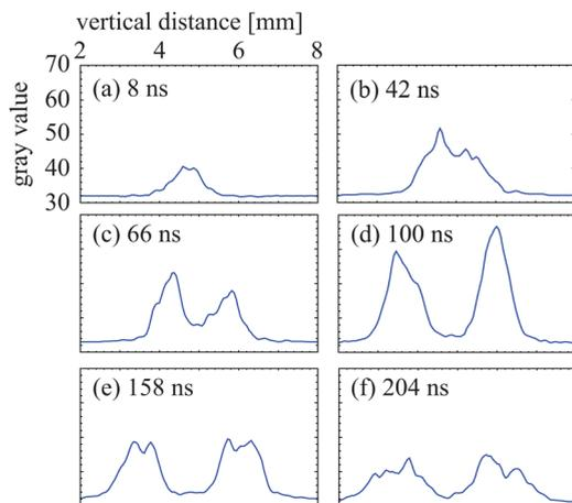
FIG. 5. (Color online) Vertical profiles of pixel intensity at fixed  $z$  in fast-gated images of breakdown with linearly polarized beam. Each frame is labeled with camera trigger time  $t$ . This sequence follows a filament born around 8 ns (a).
