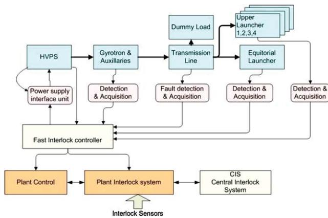
Fig. 4. A typical schema for fast interlock processing for EC system.
