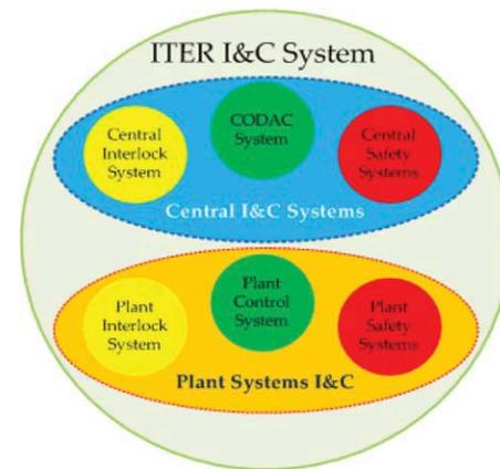
Fig. 2. ITER instrumentation and control components and its organization.
