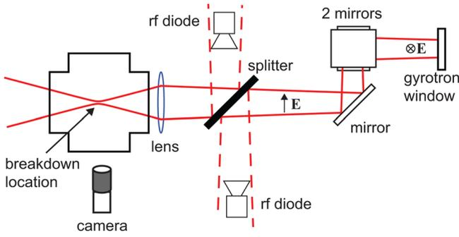
FIG. 1. (Color online) Experimental setup for breakdown delay time measurements.
