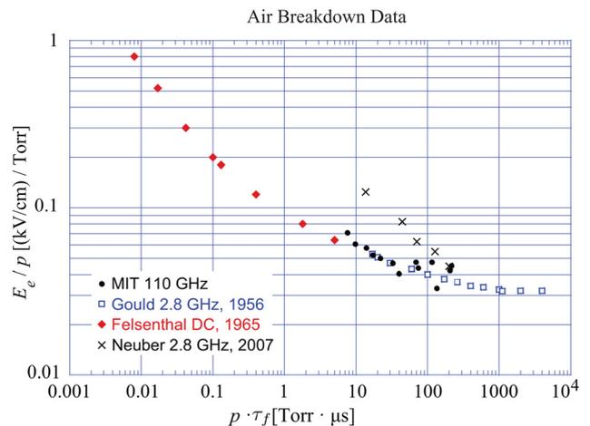
FIG. 5. (Color online) Comparison of breakdown time and field amplitude data between the present 110 GHz experiment (black circles), Gould *et al.*<sup>27</sup> (open squares), Felsenthal *et al.*<sup>28</sup> (red diamonds), and Neuber *et al.*<sup>29</sup> (black crosses).
