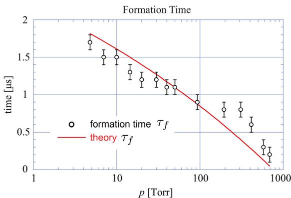
FIG. 4. (Color online) Measured formation time (open circles) versus pressure. The solid red curve is calculated from the formative time distribution theory of Eq. (8)
