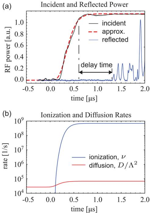
FIG. 2. (Color online) (a) Measured incident power waveform (solid black line) with analytical approximation (dashed red) and normalized reflected power (solid blue). (b) Ionization and diffusion loss rates at 700 Torr during the rise of the microwave pulse, calculated with empirical expressions and  $E_{rms}(t)$ .
