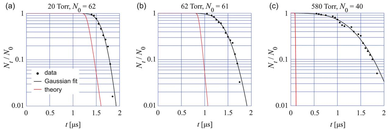
FIG. 3. (Color online) Number of events  $N_t$  observed after time  $t$  (black circles), as a fraction of total measurement number  $N_0$ , at (a) 20 Torr, (b) 62 Torr, and (c) 580 Torr. The solid black curves are Gaussian probability distribution fits to the data. The solid red curves are the theoretical formative distribution of Eq. (8).
