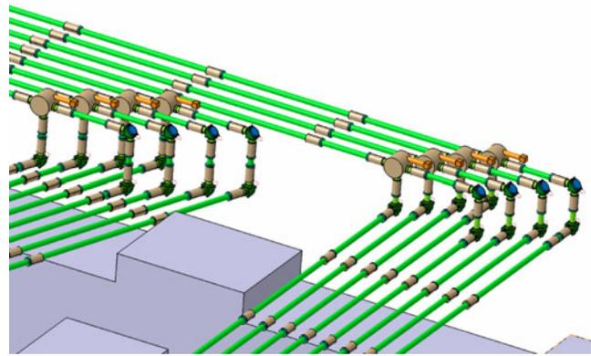
Fig. 7. TL connections toward ports 12 and 13 upper launchers.
