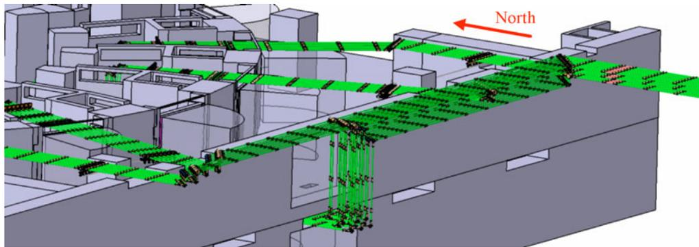
Fig. 4. TL routing along south tokamak wall and connections to upper port launchers.
