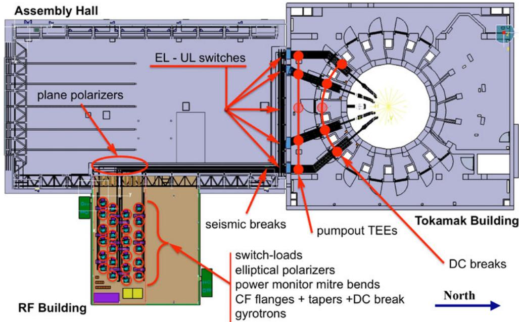
Fig. 2. EC H&CD system layout and TL components' location.
