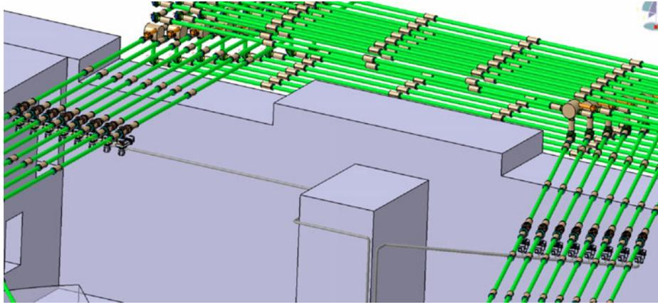
Fig. 8. New pump-out tee location close to tokamak building penetrations.
