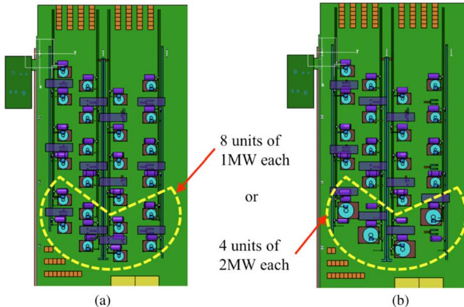
Fig. 9. Alternative layouts in the rf building for the European sources: (a) eight 1-MW units and (b) four 2-MW units.
