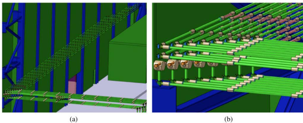
Fig. 5. (a) TL layout on the east assembly hall wall and (b) detail of the switches to port 16 upper launcher.
