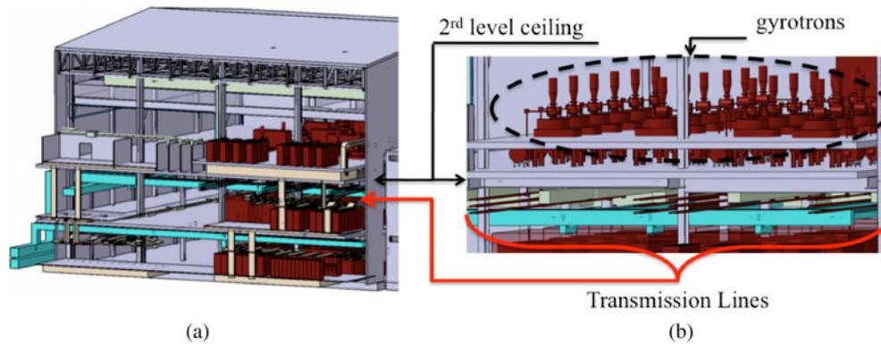
Fig. 3. (a) EC components' arrangement in the rf building at the intersection with assembly hall (not showed in the figure) and (b) detail of the TL routing under the ceiling of the second level.
