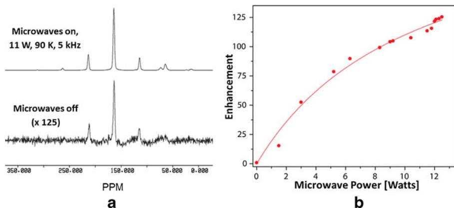
**Fig. 8** a) Enhancement spectra for  $^{13}\text{C}$ -Urea dissolved in a 60/30/10 glycerol/ $\text{D}_2\text{O}/\text{H}_2\text{O}$  glass forming matrix containing 10 mM TOTAPOL and 5 kHz spinning frequency. b) Microwave power vs enhancement for the  $^{13}\text{C}$ -Urea sample.
