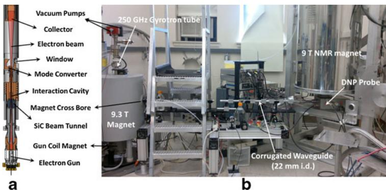
**Fig. 1** a) Drawing view of the frequency-tunable 250 GHz gyrotron. b) Gyrotron in a 9.3 T superconducting magnet and NMR spectrometer and their related components as installed at the Francis Bitter Magnet Lab, MIT.
