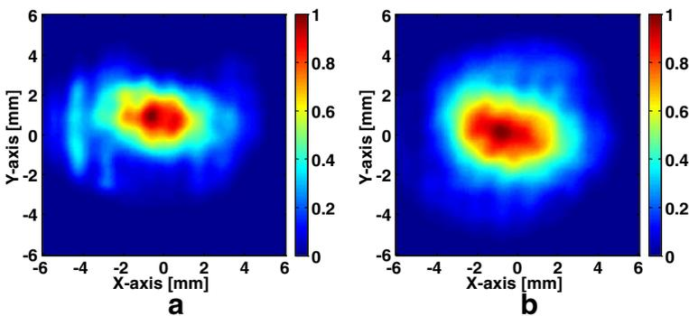
**Fig. 7** Beam profile measured using a pyrocam at 4 cm in air radiated from the waveguide aperture at 1.2 m from the gyrotron output window at two different frequencies, a) 249.18, and, b) 250.58 GHz respectively.
