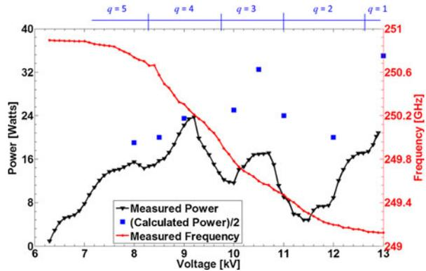
operating voltage, compared to varying the magnetic field at a constant voltage. The frequency of the radiation was measured with a heterodyne measurement system consisting of a detector diode/diplexer and a local oscillator (18 – 26 GHz range).
